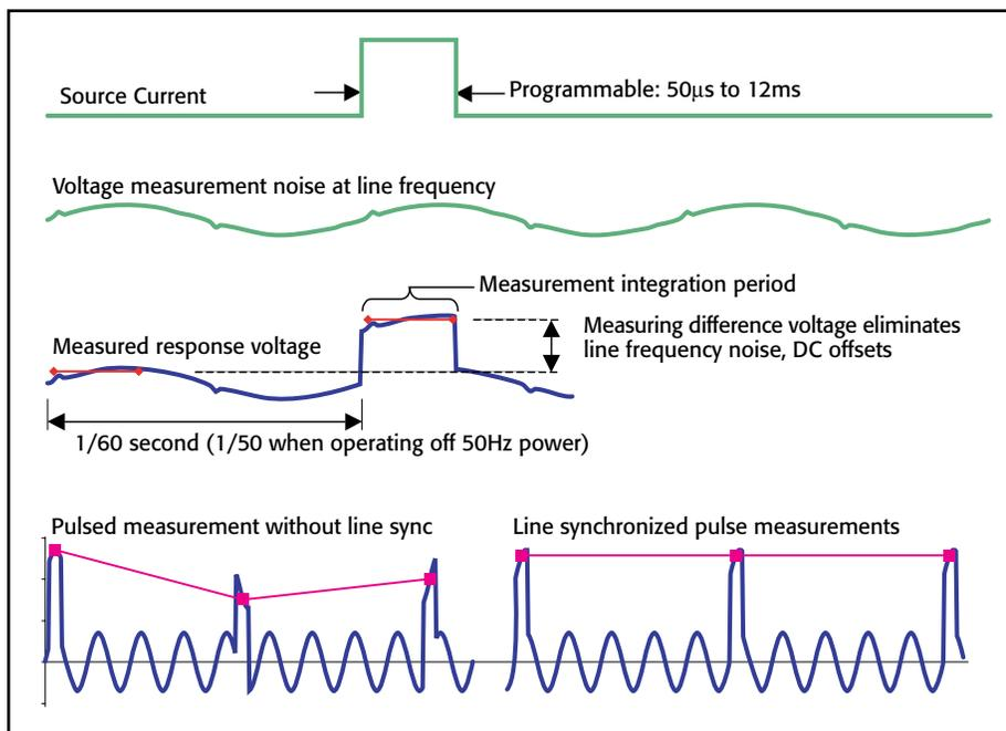
**Figure 3. Measurements are line synchronized to minimize 50/60Hz interference.**
