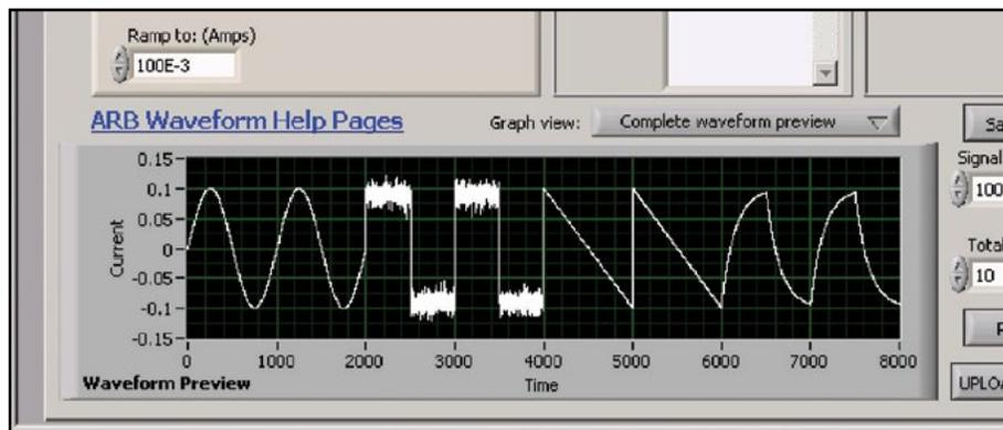
**Figure 4. The Model 6221 and the free example start-up control software make it easy to create complex waveforms by adding, multiplying, stringing together, or applying filters to standard wave shapes.**
